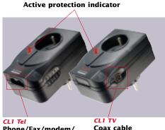
Phone/Fax/modem/ internet protection : surge suppression on phone lines to avoid hardware damage CL1 TV Coax cable protection TV/VCR/audio systems
